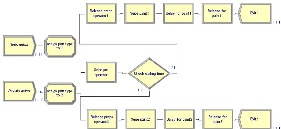
**Figure 3** Simulation of the opening channel for painting, add one channel in the Arena Simulation program.
